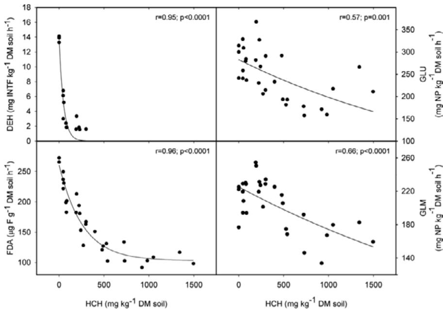
**Figure 2.** Effect of HCH concentration on soil dehydrogenase (DEH), fluorescein diacetate hydrolysis (FDA),  $\beta$ -glucosidase (GLU) and  $\beta$ -glucosaminidase (GLM) activity. INTF, iononitrotetrazolium violet-formazan; F, fluorescein sodium salt; NP, nitrophenol.
