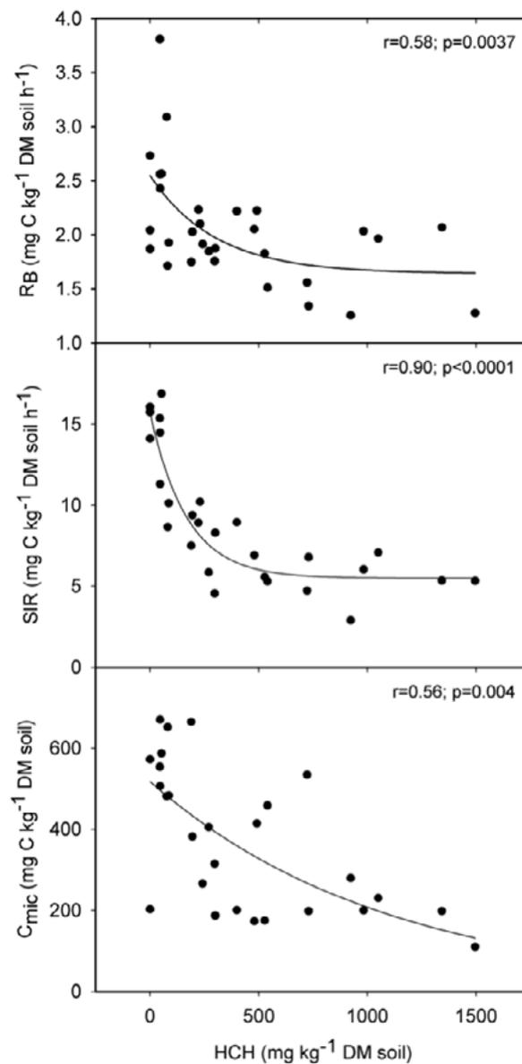
**Figure 3.** Effect of HCH concentration on soil basal respiration ( $R_B$ ), substrate-induced respiration (SIR) and microbial biomass carbon ( $C_{mic}$ ).
