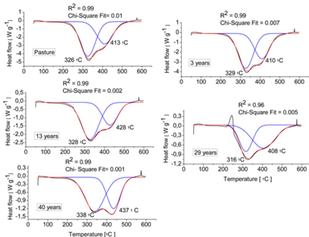
Figure 4. Results for the two peaks fit to DSC curves to monitor the variation of the peak height of both peaks in the chronosequence. Red lines represent the theoretical Gaussian curve fit. Black lines are the original DSC curves. Blue lines are the deconvoluted peaks. Each plot shows the correlation coefficient and the Chi-Square fit values of the curves adjustment, together with the temperatures of the deconvoluted peaks.
