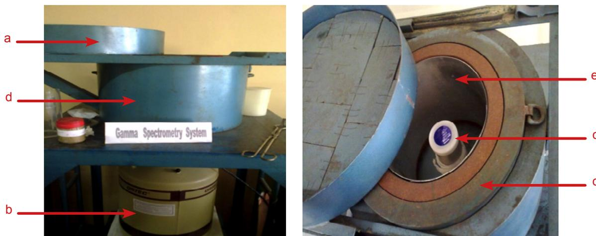
**Figure 2.** A coaxial high purity germanium (HPGe) detector and a set of shielding (a) door closed tightly against shield body (b) liquid nitrogen cryostat (c) detector located near center of shield volume (d) cylindrical lead material and (e) an inner layer of copper.
