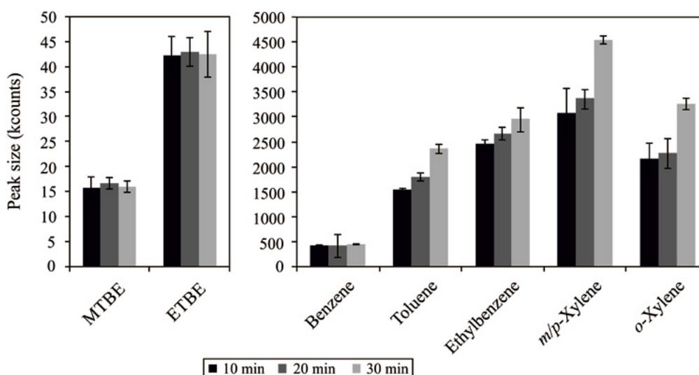
**Figure 6.** Peak sizes of individual FO and BTEX in  $500 \mu\text{g L}^{-1}$  water standards analyzed by HS-SPME-GC-MS, at different incubation times.
