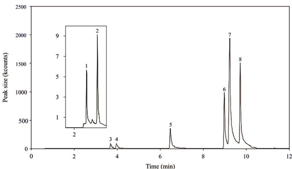
**Figure 8.** Example of a HS-SPME-GC-MS chromatogram of a 2500 µg L<sup>-1</sup> water standard. The peaks correspond to MTBE (1), ETBE (2), benzene (3), fluorobenzene (4), toluene (5), ethylbenzene (6), *m/p*-xylene (7) and *o*-xylene (8).
