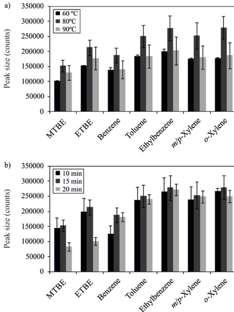
**Figure 2.** Peak sizes of individual FO and BTEX in 500  $\mu\text{g L}^{-1}$  water standards analyzed by HS-GC-MS, at different incubation temperatures (a) and times (b).
