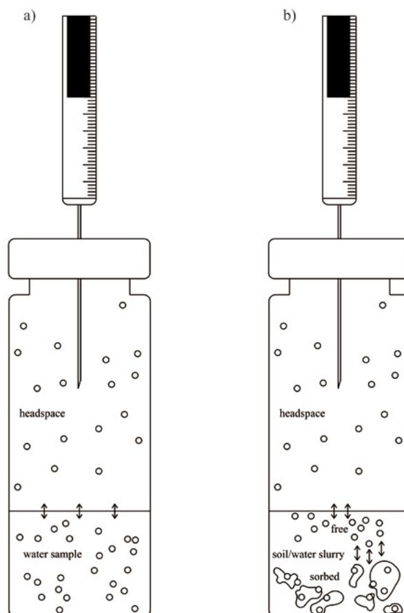
**Figure 1.** Simplification of equilibrium processes occurring in VOA vials with water (a) and soil (b) samples during HS analysis.
