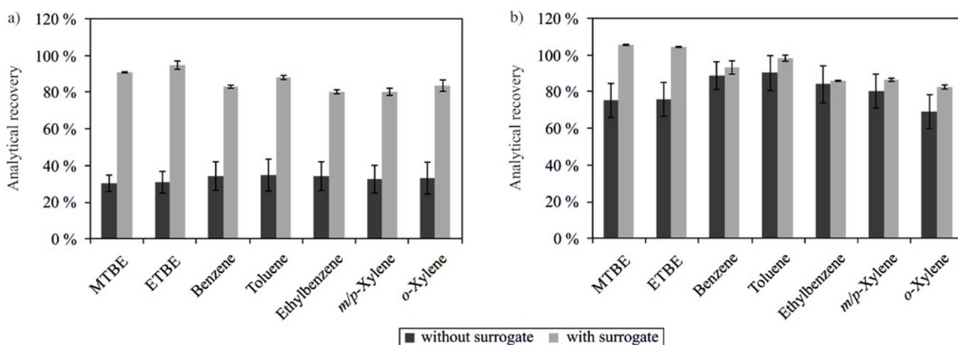
**Figure 4.** Analytical recoveries of individual FO and BTEX from  $A_{\text{Camb}}$  (a) and  $B_{\text{Camb}}$  (b) spiked with  $1000 \text{ µg kg}^{-1}$  and analyzed by HS-GC-MS without and with the addition of surrogate (fluorobenzene,  $5000 \text{ µg kg}^{-1}$ ).
