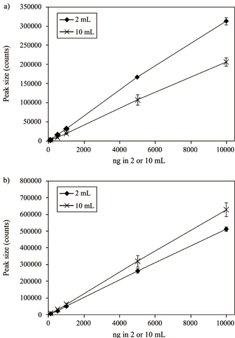
**Figure 3.** Examples of peak sizes of ETBE (a) and ethylbenzene (b) resulting from HS-GC-MS analysis of 2 mL and 10 mL standards.
