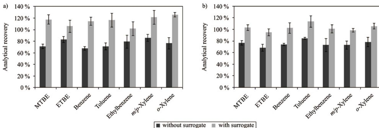
**Figure 7.** Analytical recoveries of individual FO and BTEX from  $A_{\text{Camb}}$  (a) and  $B_{\text{Camb}}$  (b) spiked with  $1000 \mu\text{g kg}^{-1}$  and analyzed by HS-SPME-GC-MS without and with the addition of surrogate (fluorobenzene,  $5000 \mu\text{g kg}^{-1}$ ).
