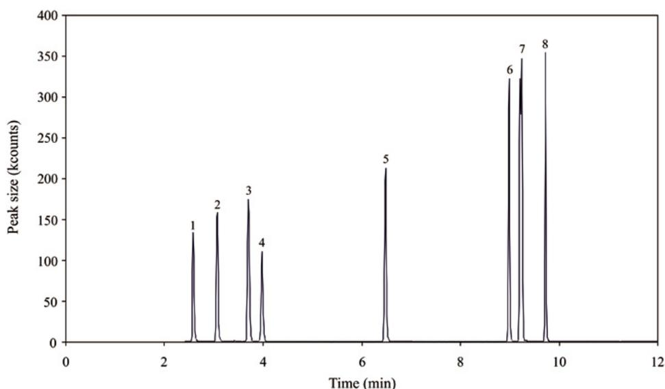
**Figure 5.** Example of a HS-GC-MS chromatogram of a 5000 µg L<sup>-1</sup> water standard. The peaks correspond to MTBE (1), ETBE (2), benzene (3), fluorobenzene (4), toluene (5), ethylbenzene (6), *m/p*-xylene (7) and *o*-xylene (8).
